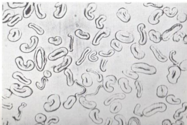
Fig. 47. Cotton, raw, Tanguis. Whole mount \times 200 . These fibres show more or less pronounced convolutions.
