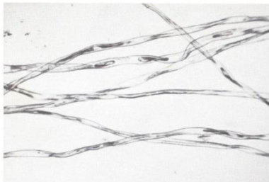
Fig. 47. Cotton, raw, Tanguis. Whole mount \times 200 . These fibres show more or less pronounced convolutions.
